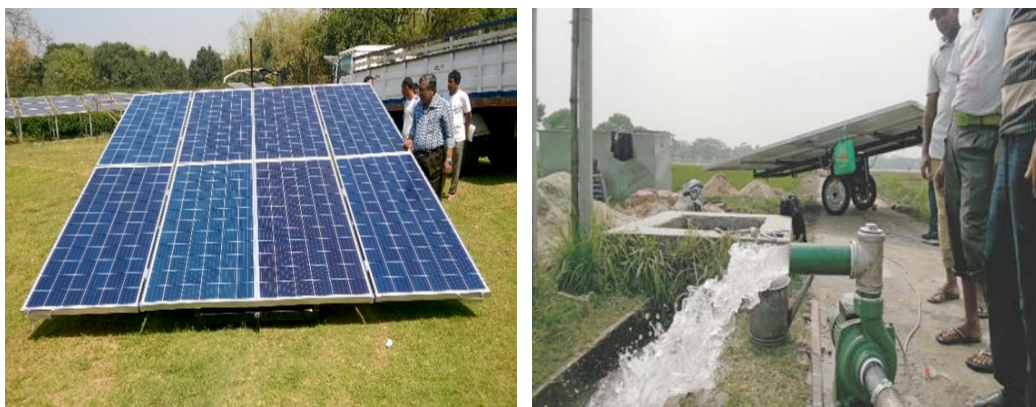
Fig. 60 Portable solar pump irrigation system
