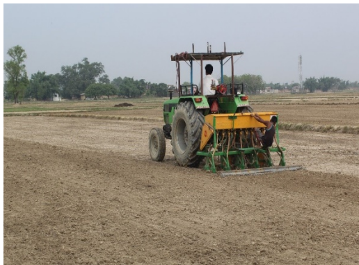
Fig. 12. Dry-DSR using tractor mounted drill.
