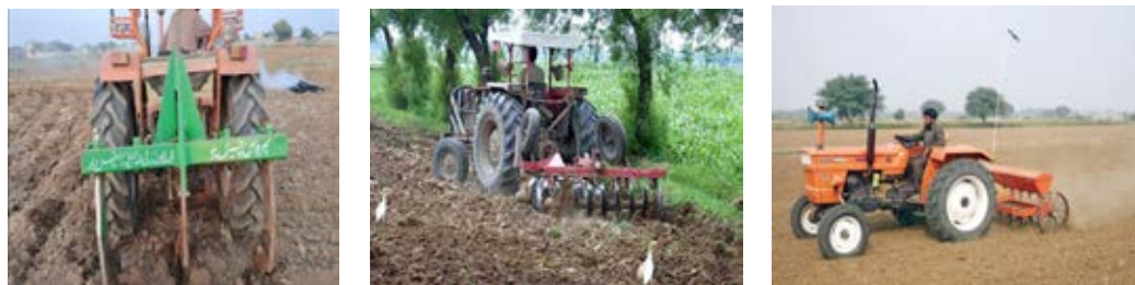
Fig. 34 Deep-tillage by using Chisel plow /Disk plow in rainfed areas
