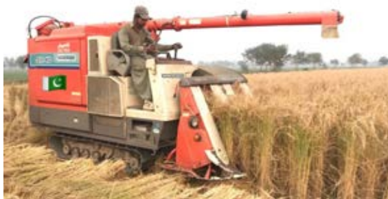
Fig. 14 Harvesting of rice crop with Kubota Combine Harvester
