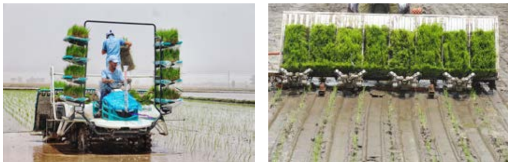
Fig. 9 Mechanical transplanting of rice
