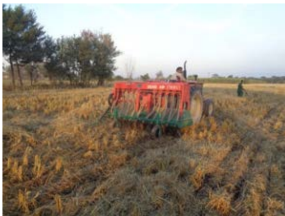
Fig. 28. Sowing of wheat crop by using Happy seeder after rice crop
