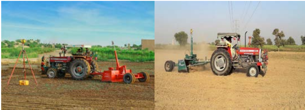
Fig. 3. Laser land leveling in the field
